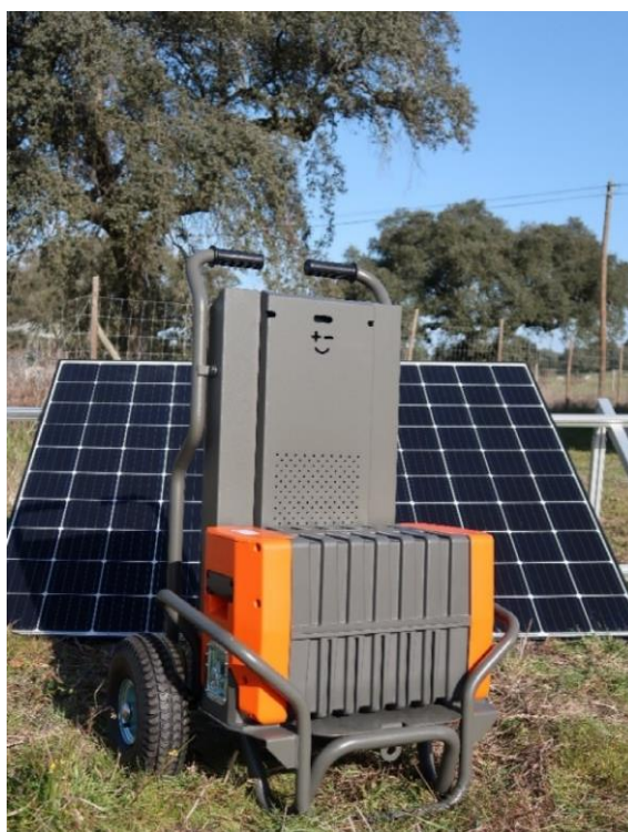
Figure 10 Demonstration of modular 2 nd Life Batteries system in real operation to power portable tools
